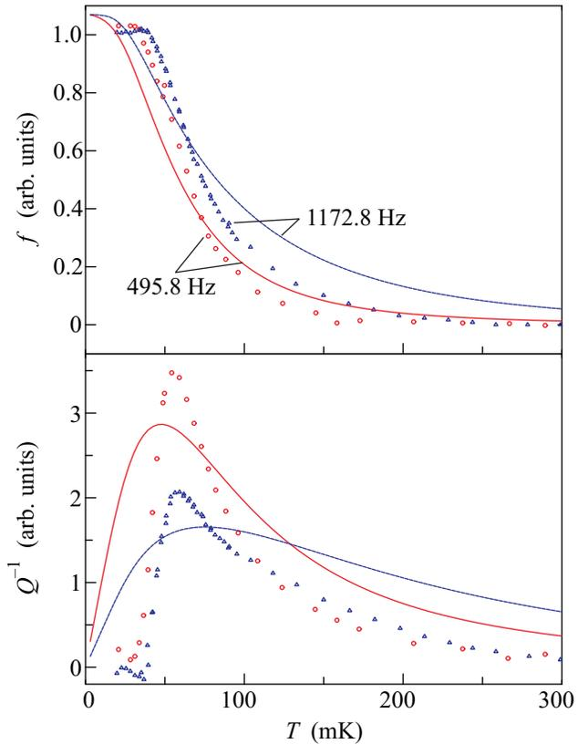
Fig.1. Temperature dependences of decoupled fraction (16) and dissipation (15) ( $\Delta = 51$  mK,  $\chi_2 = 5.9$  kHz/K) for two frequencies fitting experimental data [24]
