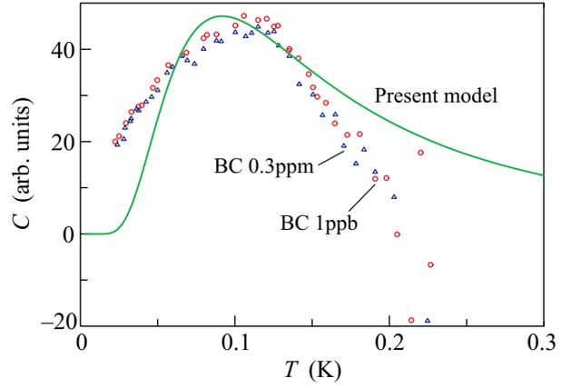
Fig. 2. Temperature dependence of heat capacity (23) ( $\Delta = 0.11$  K) and experimental data [9]
