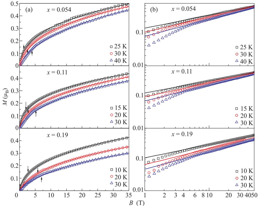
Fig. 1. (Color online) Magnetization field dependences for  $Mn_{1-x}Fe_xSi$  in the units of Bohr magneton per Mn ion. Points in the panels (a, b) – experiment, lines in the panel (b) – best fit by the power law  $M(B) \sim B^\alpha$ , lines in the panel (a) – best fit with the help of interpolating formula. Arrows in the panel (a) denote crossover fields  $B_c$ .
